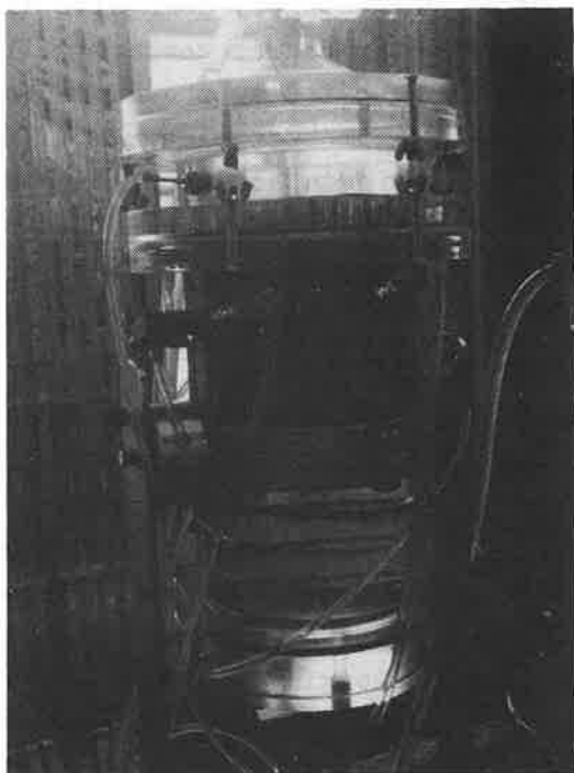
Fig. 1 A flow permeameter as used in the tests. See text for description
