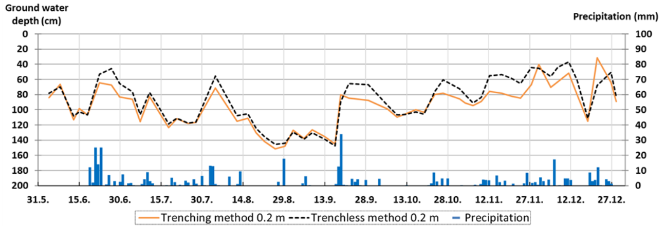
Figure 5. Groundwater table depth (average of the manual measurements; cm) at the distance of 0.2 meter from the drain and precipitation in the period 6/2015-12/2015. The average groundwater table depths represent the four field sections with the similar drainage method.
