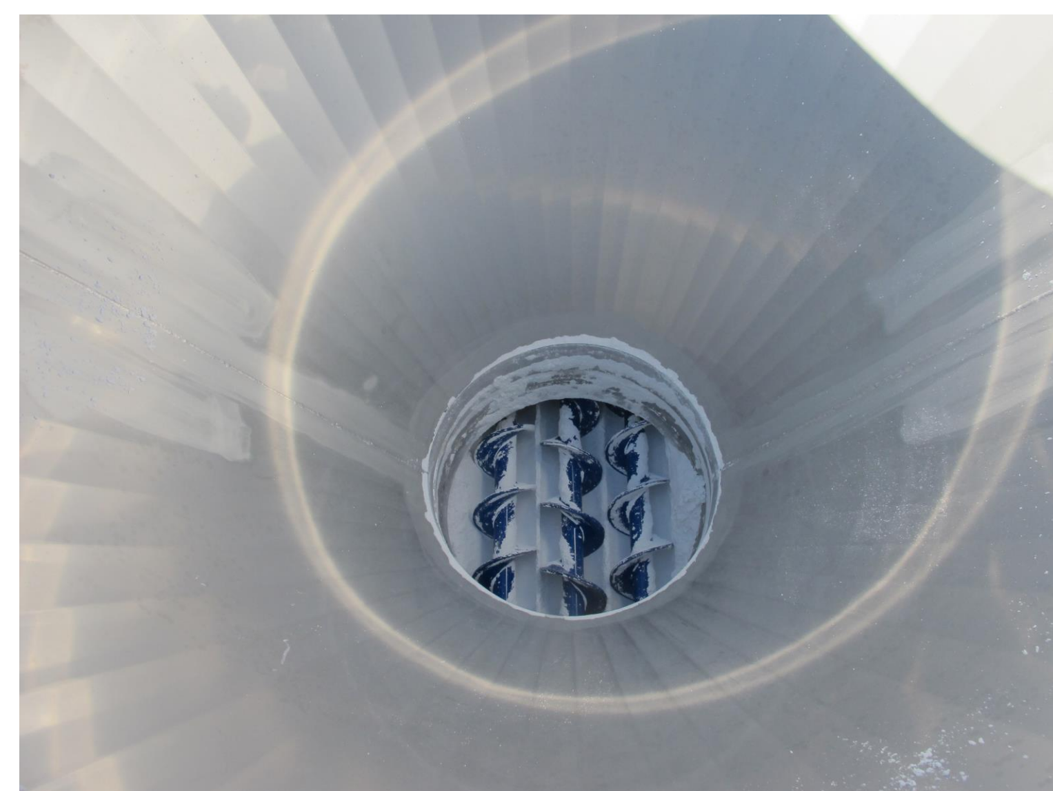
Three screws in the bottom of the funnel enables an exact dosing of the C2 powder
