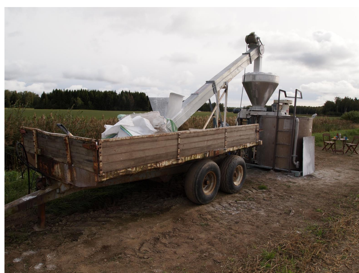
A conveyor belt is transporting the C2 powder to a funnel
